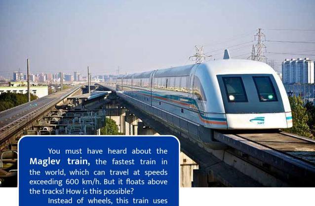
Instead of wheels, this train uses magnets, and there are also magnets on the tracks it runs on. However, these magnets are placed so that like poles face each other. This repulsion prevents the train from touching the tracks and eliminates friction, allowing the train to travel at full speed.
